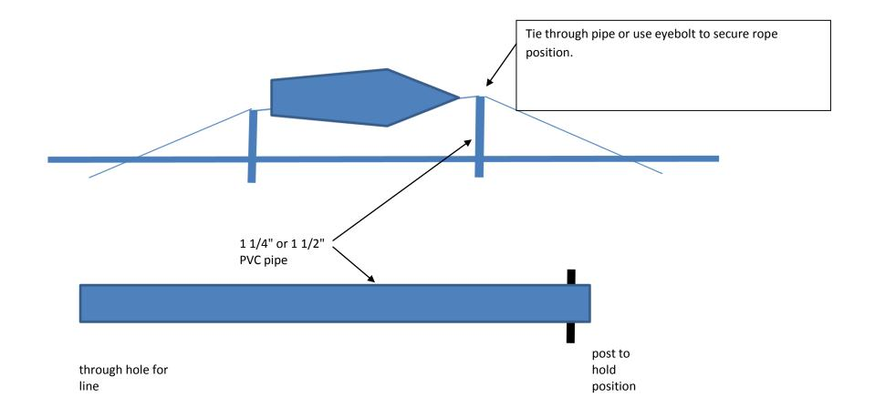
Keep ends tied to shore. To launch pull pipe off of post and pull boat close to dock. Remove hook from bow and stern eyes and stow rope and pipe on shore. To secure boat after use reattach hooks to bow and stern eyes and use pipe to push out and tighten rope.
