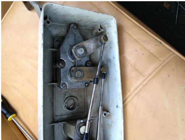
Forward (Fast Idle) but Hitting Stops, Still Neutral – Should be able to throttle up a bit here but hitting stops first.
