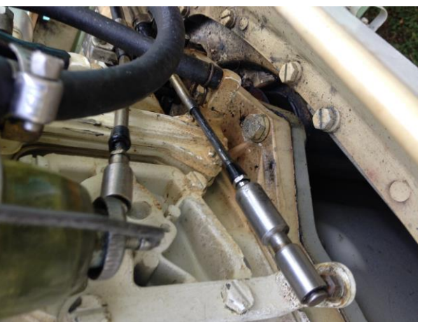
Forward (Fast Idle) but Hitting Stops, Still Neutral – Should be able to throttle up a bit here but hitting stops first.
